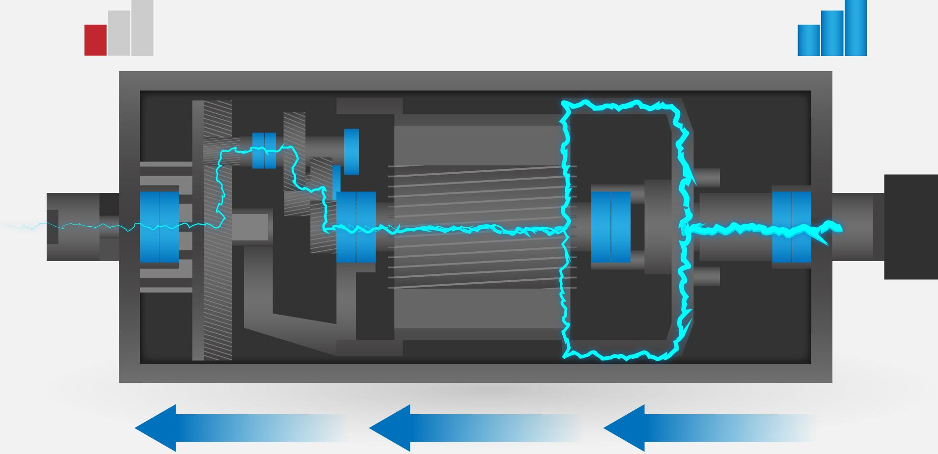
Electrical energy is lost as it passes through each rotating component of the drum motor.
