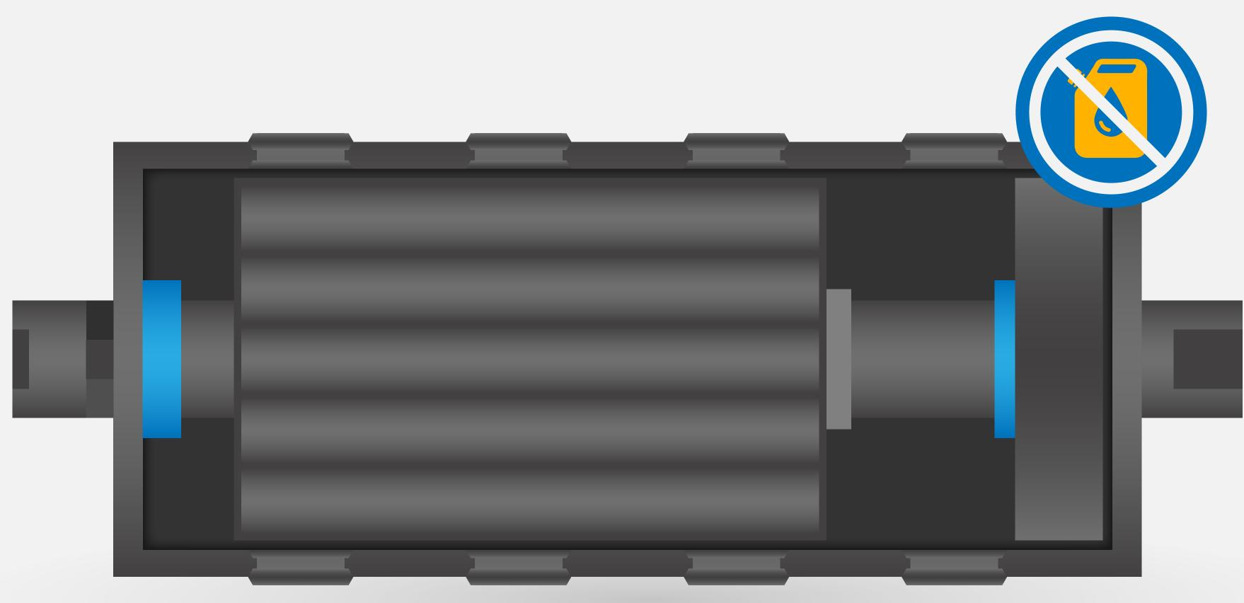
Mag-drives on the other hand are lubricant free, which means there is no oil used above the food line. No Oil. No threat of oil leak!
