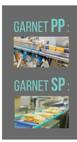
Ensures precise product alignment, ideal for handling grouped products in optimizing processes in **primary packaging**. It automates the arrangement of products into a single file, repositioning and phasing them to the infeed section of a flow wrapper. Whether it's delicate, irregularly shaped, or varying size items,
